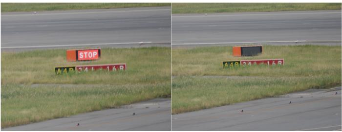
Figure 1: On left, Variable Message Sign displays "Stop". On right, Variable Message Sign off.
